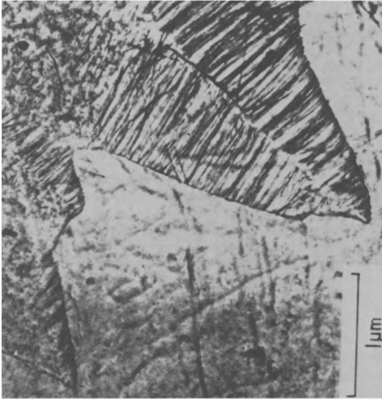
Fig. 5.71 Fe-4% Mo-0.2% C transformed 2 h at 650 °C. (a) Schematic of possible nucleation and growth mechanism. (b) Thin foil electron micrograph ( \times 32\,000 ) (after R.W.K. Honeycombe, 'Transformation from Austenite in Alloy Steels', Metallurgical Transactions , 7A (1976) 91, © American Society for Metals and The Metallurgical Society of AIME, 1976, after D.V. Edmonds.)
