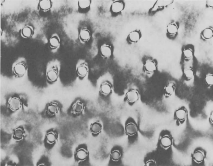
Fig. 4.30 Rod-like eutectic. \text{Al}_6\text{Fe} rods in Al matrix. Transverse section. Transmission electron micrograph ( \times 70\,000 ). (Courtesy of J. Strid, University of Luleå, Sweden.)
