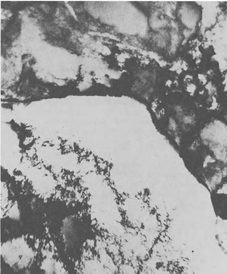
Fig. 3.26 Grain boundary migration in nickel pulled 10% and annealed 10 min at 425 °C. The region behind the advancing boundary is dislocation-free. (After J. Bailey and P. Hirsch, Proceedings of the Royal Society , London, A267 (1962) 11.)
