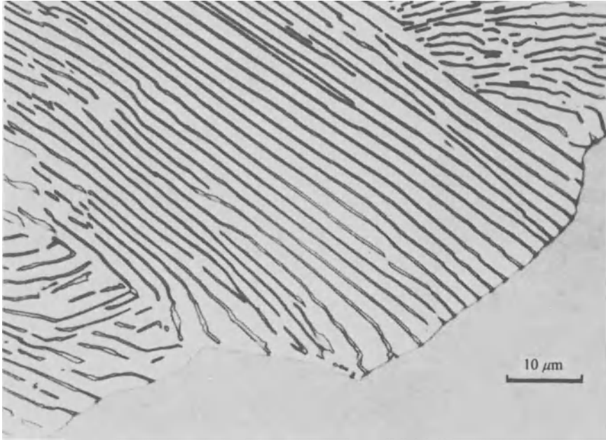
Fig. 5.55 A pearlite colony advancing into an austenite grain. (After L.S. Darken and R.M. Fisher in Decomposition of Austenite by Diffusional Processes , V.F. Zackay and H.I. Aaronson (Eds.), by permission of The Metallurgical Society of AIME.)
