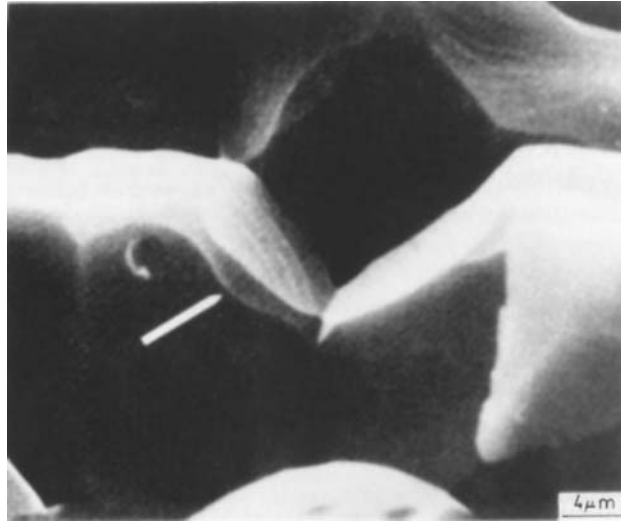
FIGURE 11.3 Scanning electron micrograph of pore channels in MgO with well-defined perturbations (arrowed). (From Ref. 12.)
